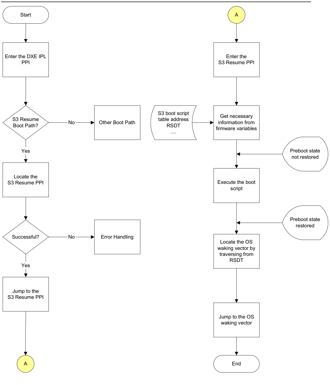
Figure 2-4. DXE IPL PPI and S3 Resume PPI in S3 Resume Boot Path
